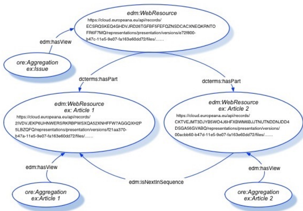
Figure 7. Representation of hierarchical relationships between a Journal Issue and its articles. Note that in this example the URIs don't correspond to URIs to real resources. More details are available in Annex 2.
